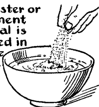
Fig. 2. Proper method for mixing plaster of Paris.
