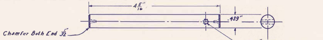
No. 9 - BULL GEAR SHAFT One. Finish all over. Stock 1" Dia. x 5 3/2" Long C.R.S.
